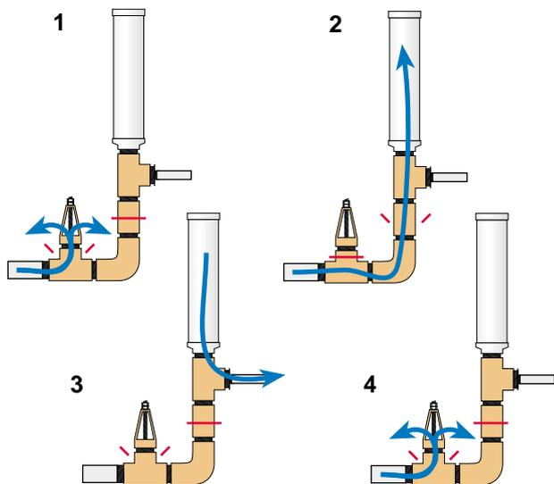
quickly than without the standpipe. Basically, a standpipe allows the ram to operate as if it had a shorter drive pipe.
