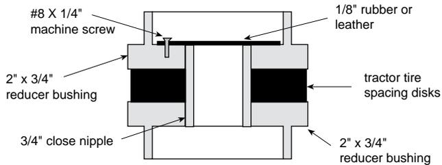
ability of the valve. This washer should be centered over and cover the width of the seat, and can be secured with a short bolt and locknut, with a small washer on the underside.
