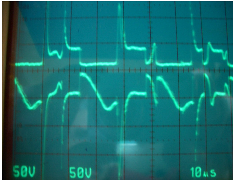
Fig. 34 (06.01.2007 - 14:39) Signals on load leads - conversion @max
