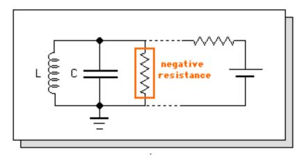
By simple circuit analysis, it is a straightforword proposition to find the following simple circuit equation which is the fundamental van der Pol oscillator equation:
